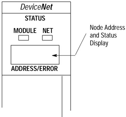
Your module uses numeric displays to indicate diagnostic information about the status of your module. The display flashes at 1 second intervals. The following table summarizes the meanings of the numeric codes.
