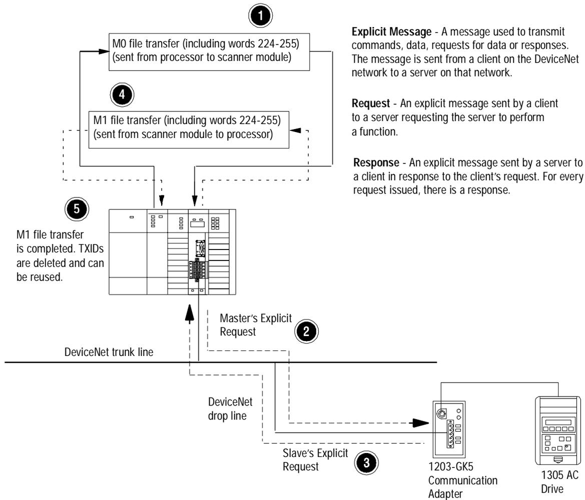
1. Format an M0 file transfer in the processor to send an Explicit Message Request to the scanner module (**download**).
