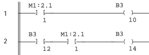
XIC instructions in rungs 1 and 2 are addressed to the M1 data file. Each of these instructions adds approximately 1ms to the scan time (5/02, Series B processor)
