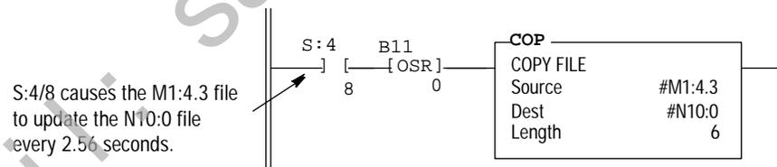
In this example, a COP instruction can be used to monitor the contents of an M1 file. When the instruction goes true, the six words of data in file #M1:4.3 is captured as it exists at that time and placed in file #N10:0. All subsequent logic should address the data in #N10:0. The data will be consistent and it shortens scan time by eliminating reads to the module each time an M0 or M1 address is encountered in the program.
