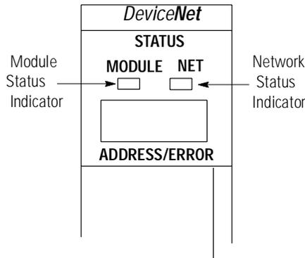
The bicolor (green/red) module status indicator (MODULE) displays module status. It indicates whether the module has power and is functioning properly.
