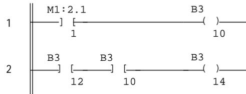
These rungs provide equivalent operation to those of the previous diagram by substituting XIC instruction B3/10 for XIC instruction M1:2.1/1 in rung 2. Scan time is reduced by approximately 1ms (5/02 Series B processor).
