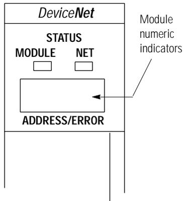
When you apply chassis power, the module numeric indicators cycle through the following displays:
